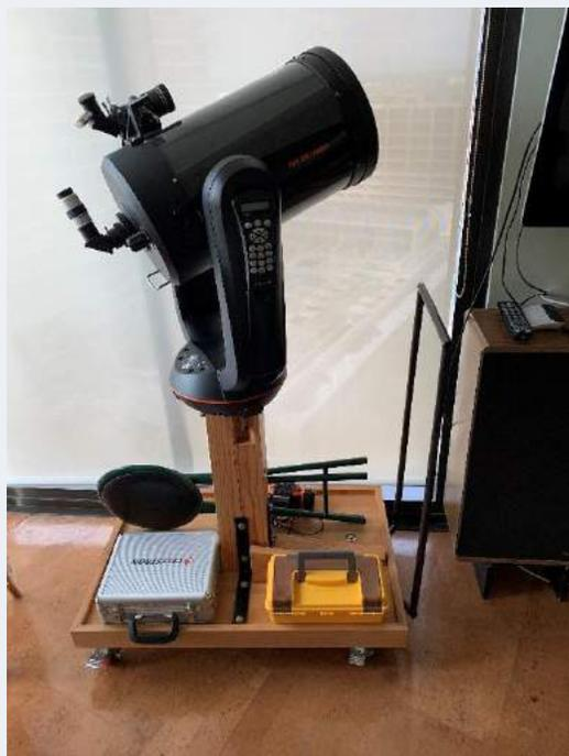
The plinth is set into a mortised opening and is held by "L" brackets. A Starizona Landing Pad is attached to the top of the plinth by countersunk wood screws and a drift pin sits in the middle, providing a target for the 'scope. The Starizona-provided attachment bolts, along with flat washers provide a stable and secure method for attaching the 'scope. With the Optical Tube angled up at 45 degrees, the assembly stands about 67" high. It rolls easily on ball
